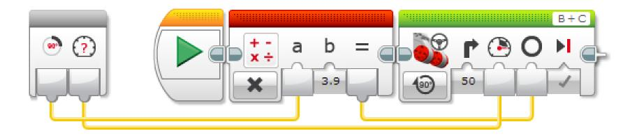
C. Wire the inputs in the grey block. The degrees input connects to the Math Block. The power goes into the Move Steering Block's power input. The result of the Math Block is wired into the Move Steering Block's degree input.
