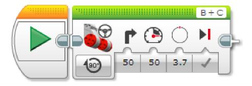
3.7 is the number of motor degrees in 1 protractor degree for Droid Bot. You will have to customize this based on your robot using Step 1A in the Powerpoint instructions.
