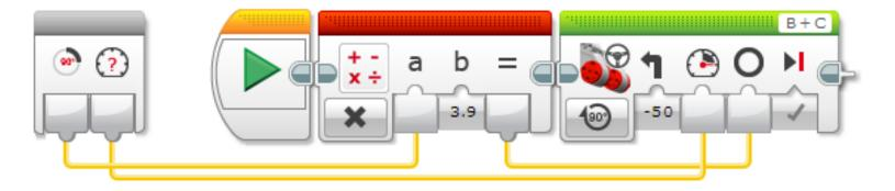
This my block converts protractor degrees to motor degrees. We turn the motor for the amount of degrees that was calculated in the previous block.
