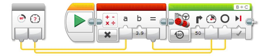
This block converts protractor degrees to motor degrees. We turn the motor for the amount of degrees that was calculated in the previous block.
